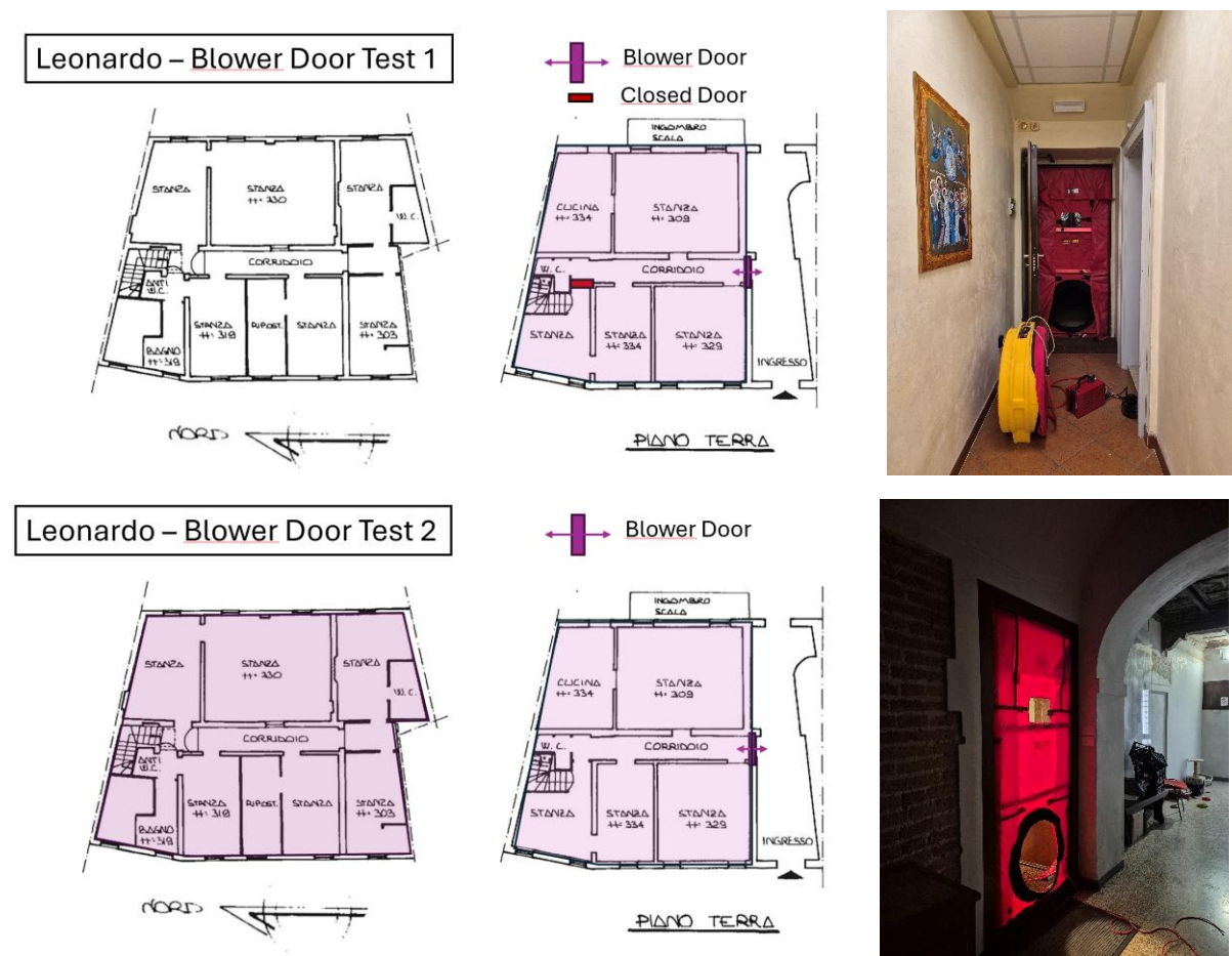
Figure 7-2: Blower Door test at Leonardo . First on ground level with door closed ( n_{50}=3,9 1/h) then on the overall building ( n_{50}=4.7 1/h).
