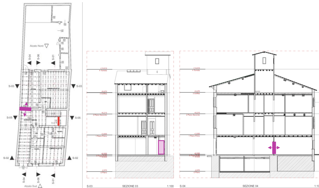
Figure 7-5: position of blower door and sealing of opening towards the cellar at Montanara .
