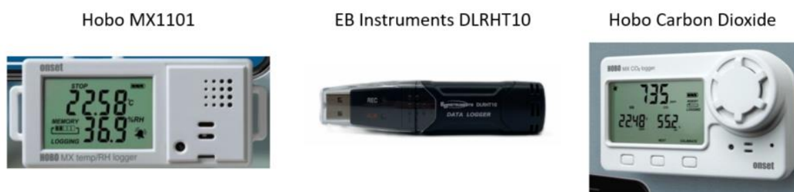
Figure 5-5 Types of datalogger adopted in the monitoring campaign.
