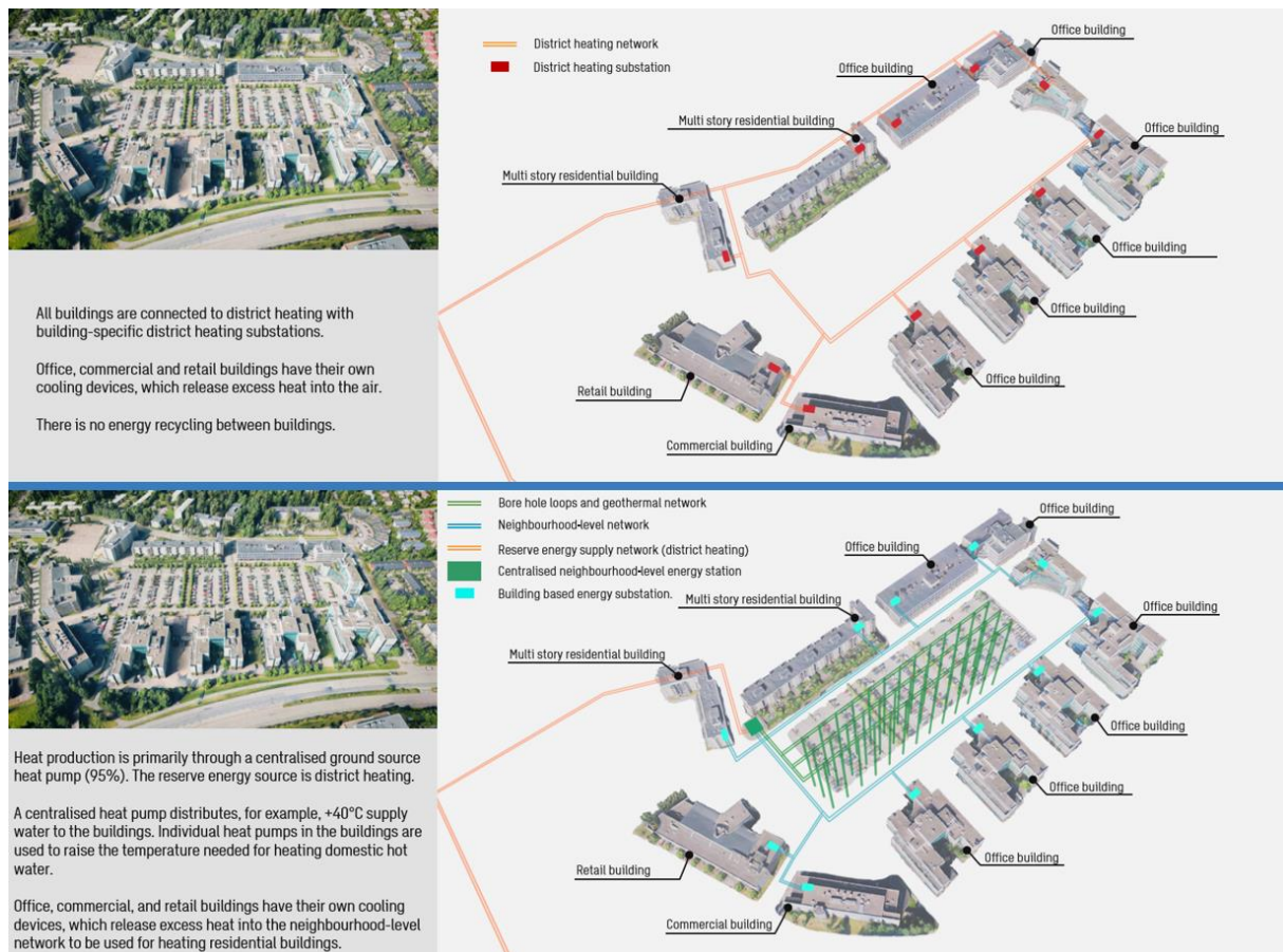
Figure 11: Above, all buildings are connected to a district heating network. Below, an example of a neighbourhood-level small thermal heating network system utilising geothermal energy and enabling the use of excess heat between buildings (Nöjd, 2024).
