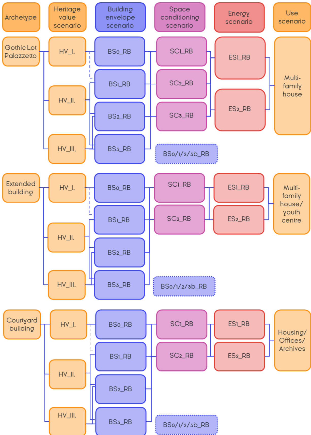
Figure 42: Overview of the renovation baseline scenarios (IT)
